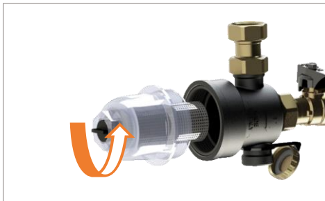
Place bucket for collecting liquid then turn anti-clockwise the glass cover using a 29 mm open wrench
